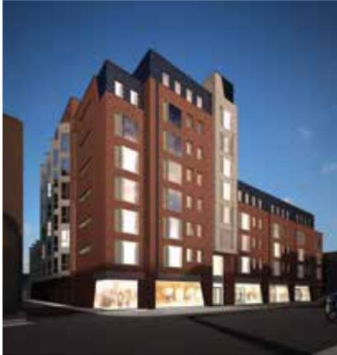
The superstructure comprises of a reinforced concrete podium slab to first floor that supports a Metframe structure to the floors above. The structure is clad in a mixture of brick work and cladding panels. Due to poor ground bearing capacity and the proximity of adjacent buildings the building's foundations are piled using CFA piles to minimise the noise and risk of vibrations damaging the adjacent properties.
