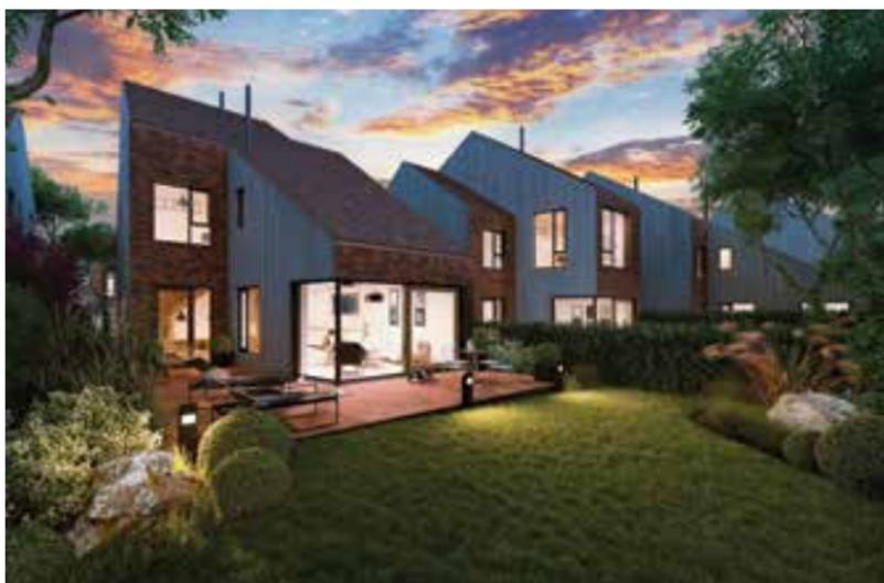
The construction of these two/three storey units is of traditional build with timber cut roofs, engineered joists and are timber brickwork clad. Additional structural steelwork has also been utilised in the design to achieve the unique architectural features. The foundations are of traditional pad and trench-fill footings at various depths to suit the topography and ground conditions.
